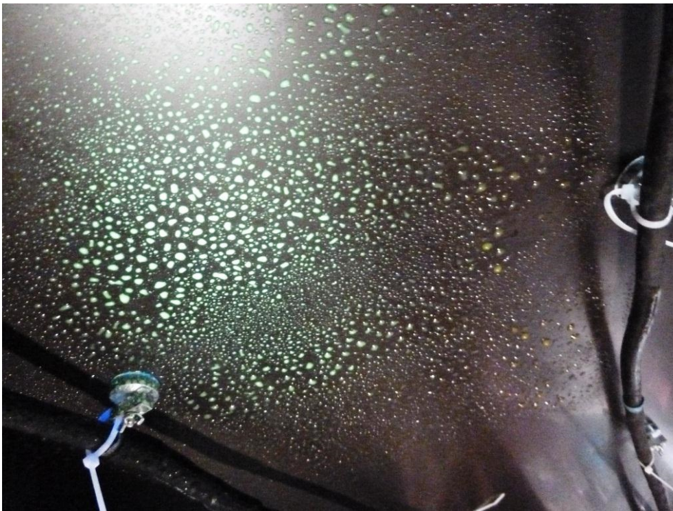
Fig. 6: no testable surface for MT (there is oil on it)
