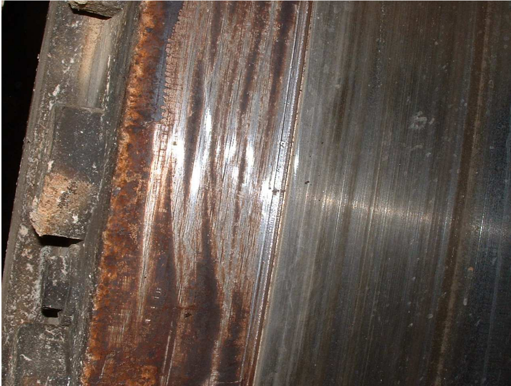
Fig. 2 : clean transition head to shell
