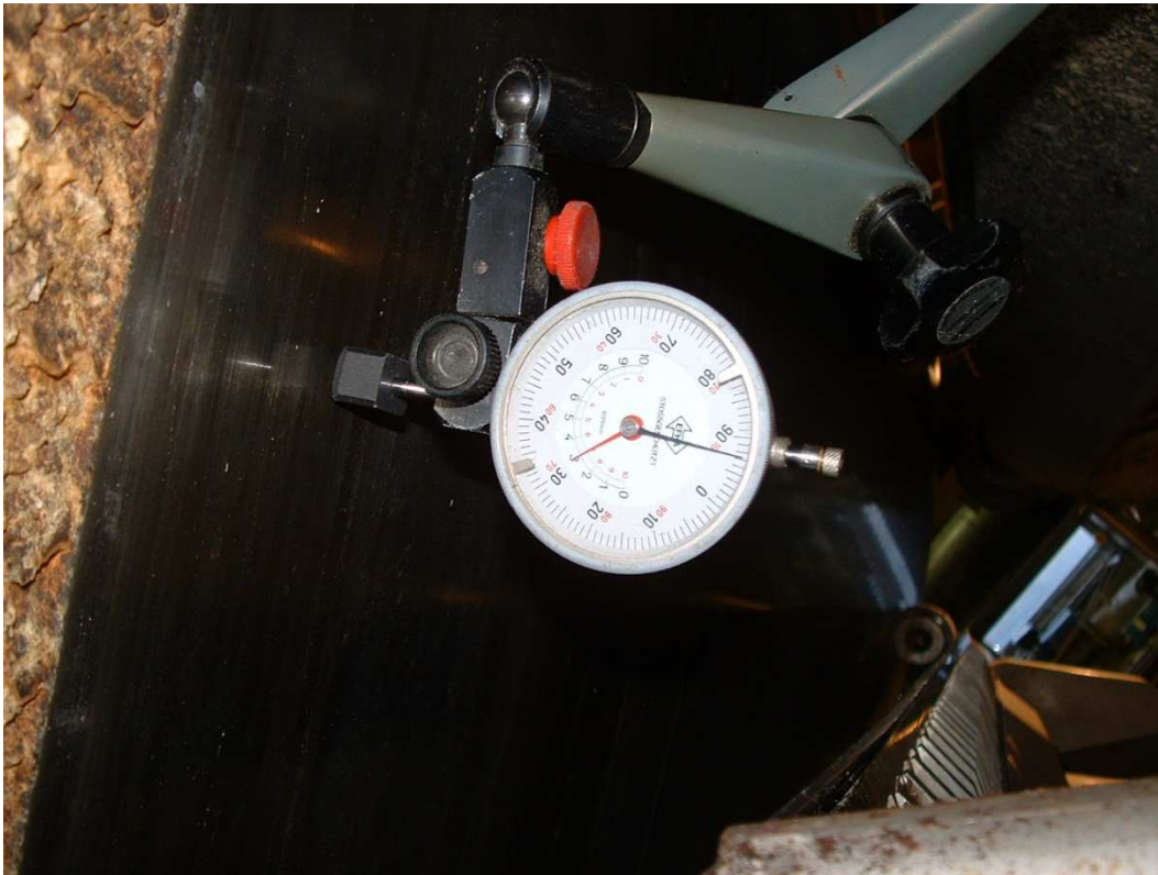
Fig. 3: a clean shell for Run Out
