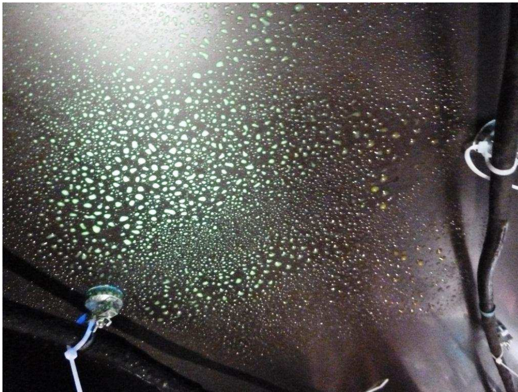
Fig. 5: surface of the shell with oil on it (not testable - MT)
